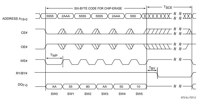
Note: This device also supports CE# controlled Chip-Erase operation. The WE# and CE# signals are interchageable as long as minimum timings are met. (See Table 13)
