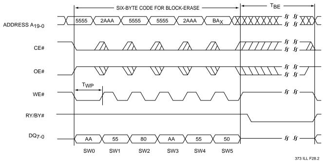
Note: This device also supports CE# controlled Block-Erase operation. The WE# and CE# signals are interchageable as long as minimum timings are met. (See Table 13)
