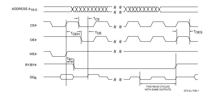
FIGURE 9: TOGGLE BIT TIMING DIAGRAM
