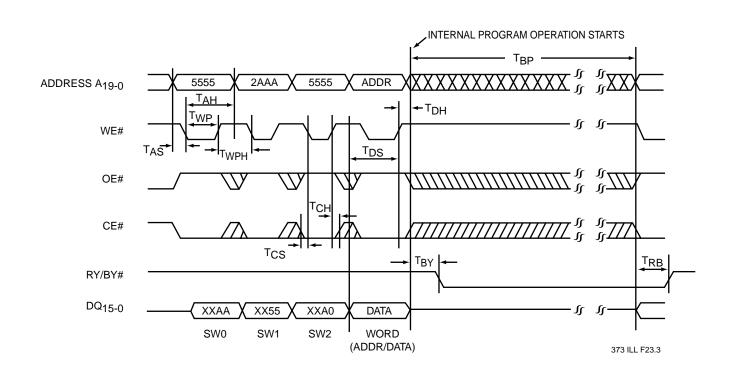
FIGURE 6: WE# CONTROLLED WORD-PROGRAM CYCLE TIMING DIAGRAM
