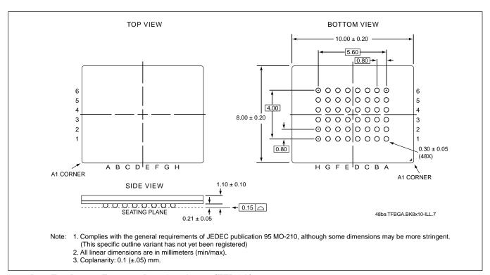
48-BALL THIN PROFILE FINE-PITCH BALL GRID ARRAY (TFBGA) 8MM x 10MM SST PACKAGE CODE: BK
