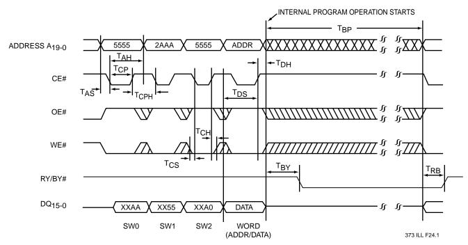
FIGURE 7: CE# CONTROLLED WORD-PROGRAM CYCLE TIMING DIAGRAM
