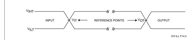
AC test inputs are driven at  $V_{IHT}$  (0.9  $V_{DD}$ ) for a logic "1" and  $V_{ILT}$  (0.1  $V_{DD}$ ) for a logic "0". Measurement reference points for inputs and outputs are  $V_{IT}$  (0.5  $V_{DD}$ ) and  $V_{OT}$  (0.5  $V_{DD}$ ). Inputs rise and fall times (10%  $\leftrightarrow$  90%) are < 5 ns.
