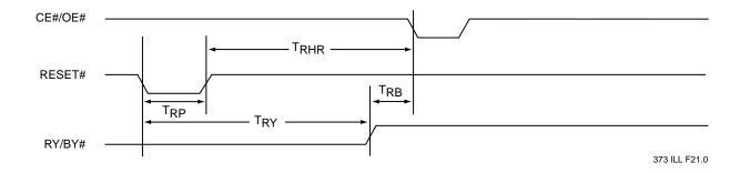
FIGURE 16: RESET# TIMING DIAGRAM
