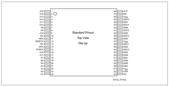
FIGURE 3: PIN ASSIGNMENTS FOR 48-PIN TSOP (12MM x 20MM)
