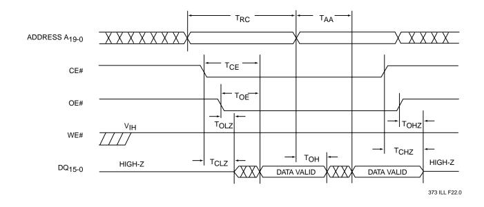
FIGURE 5: READ CYCLE TIMING DIAGRAM
