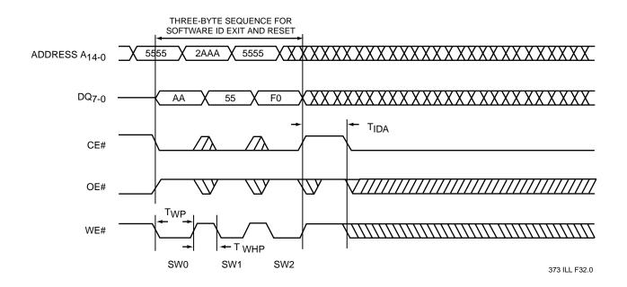
FIGURE 15: SOFTWARE ID EXIT/CFI EXIT
