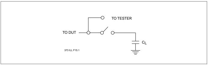
FIGURE 18: A TEST LOAD EXAMPLE
