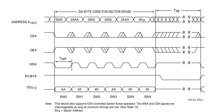
FIGURE 12: WE# CONTROLLED SECTOR-ERASE TIMING DIAGRAM
